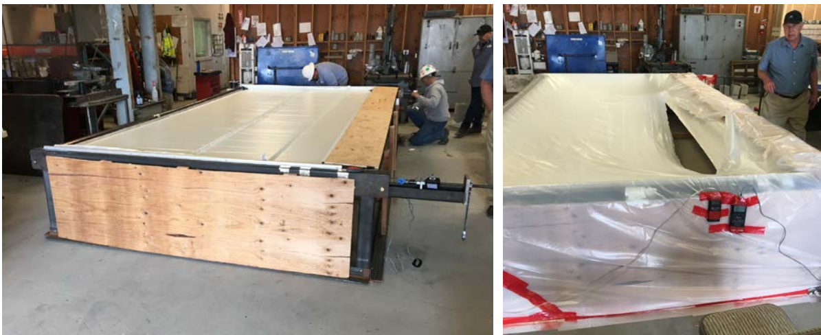
Figure 6. Vacuum chamber and zippered panel prior to testing (left), zippered panel following rupture of zipper and polyethylene cover (right)
